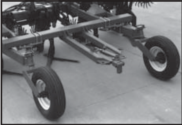
Dual Lift Assist Wheel Mounted Rear Telescoping Hitch
