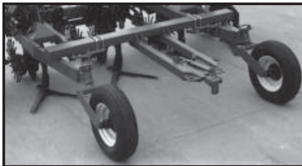
Dual Lift Assist Wheel Mounted Rear Telescoping Hitch Shown
